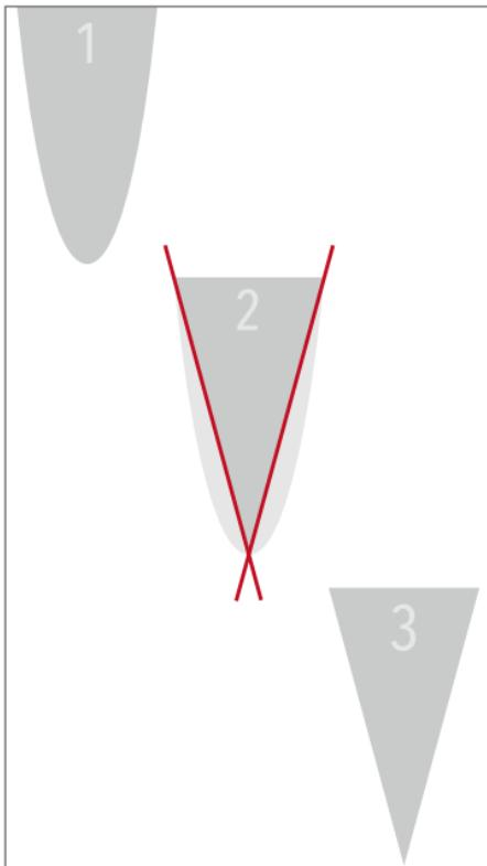
Even the best cutting tools eventually lose their sharpness. This is physics, since every metal is subject to abrasion when being used, leading to wear and rounding of the cutting edge. The principle of sharpening is hence based on taking material off the sides of the cutting edge, so as to create a new pointed tip.
