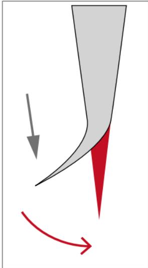
When the sharpness of a newly sharpened blade begins to fade, this usually is not due to a rounded edge, but a bent one. Here the very thin tip of the blade is slightly misaligned, so that the tip hits the cutting medium no longer in a perfect 90° angle, which is felt as reduced sharpness.
