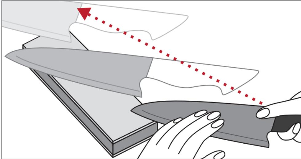
Stropping is the final step in sharpening. It refines the edge and removes the burr.
